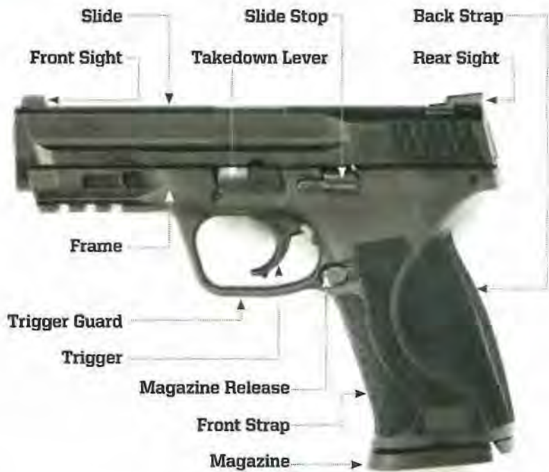
▲ Typical semi-automatic pistol, left side, with major components indicated.
